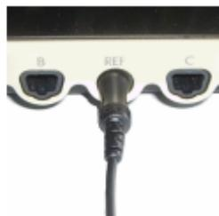
**REF** The REF port is located in the center of the channel ports at the bottom of the device.
